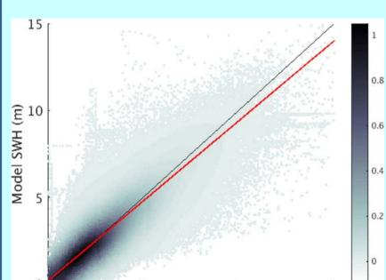
Thorough model evaluation of wave height, period, and direction is performed at 23 buoy sites around NW Europe. The model performs best in deep water, and at exposed sites. There is little improvement in wave height when downscaling, however the wave directions improve significantly. NB maximum waves are of the order twice as large as the mean significant wave heights (Hs).
