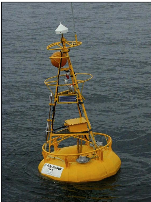
Figure 8.3 The GFZ Potsdam GPS buoy.
