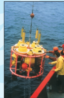
Bottom pressure sensing instrument MYRTLE, being deployed in the South Atlantic
