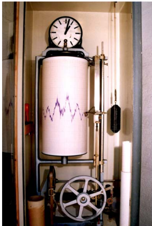
Fig. 2 Mechanical tide-gauge A. Ott – Kempten at Split.
