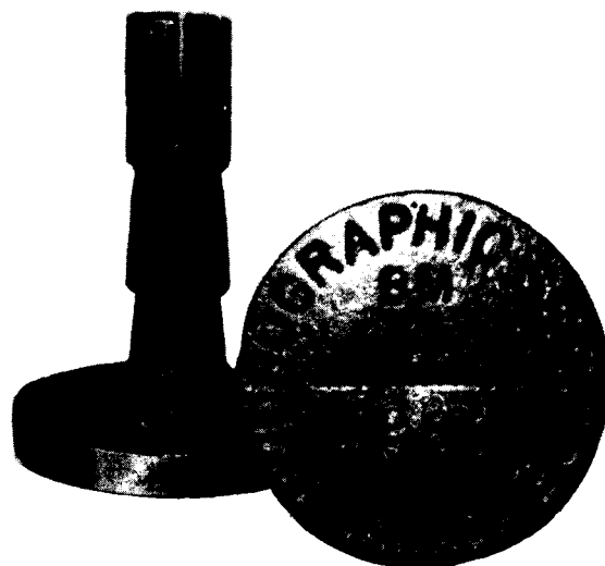
FIG. 51. Standard Canadian Hydrographic Service benchmark tablet.
